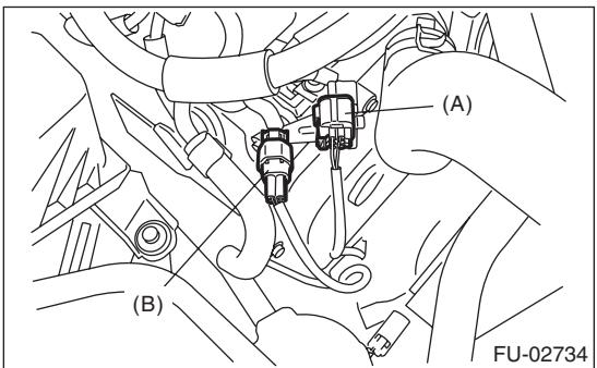
(A) Front oxygen (A/F) sensor connector
