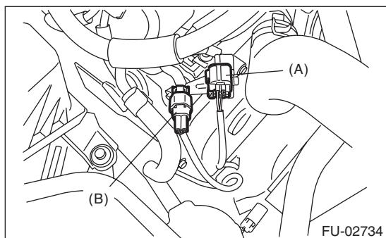
(A) Front oxygen (A/F) sensor connector
