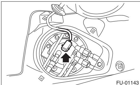
7) Disconnect the quick connector, then disconnect the fuel delivery hose, return hose and jet pump hose. <Ref. to FU(H4DOTC)-67, REMOVAL, Fuel Delivery, Return and Evaporation Lines.>
