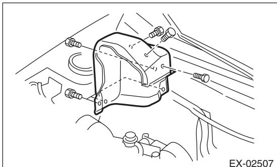
16) Install the intercooler bracket RH.
