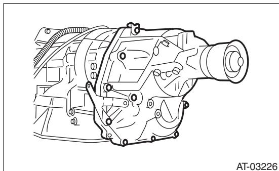
4) Remove the center differential carrier. <Ref. to 5AT-73, REMOVAL, Center Differential Carrier.>
