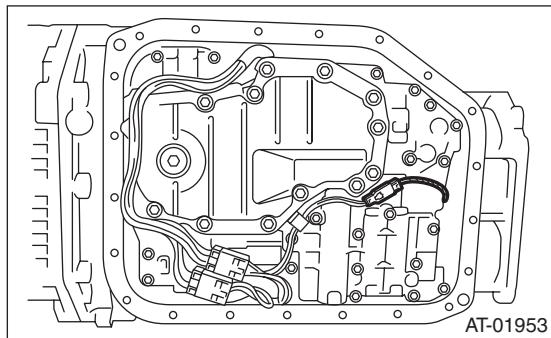
8) Remove the front vehicle speed sensor securing bolt.
