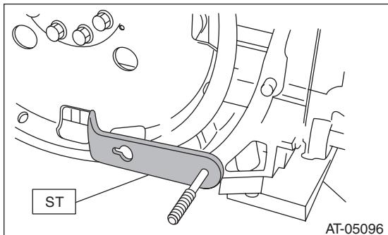
3) Tighten the drive plate in three stages. (turbo model)
