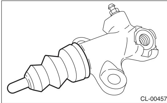
2) Apply compressed air through clutch hose attaching port.
