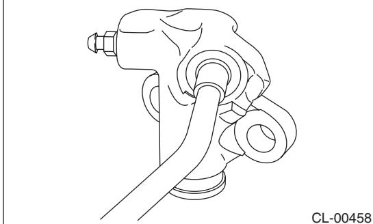
3) Separate the piston and piston spring.
