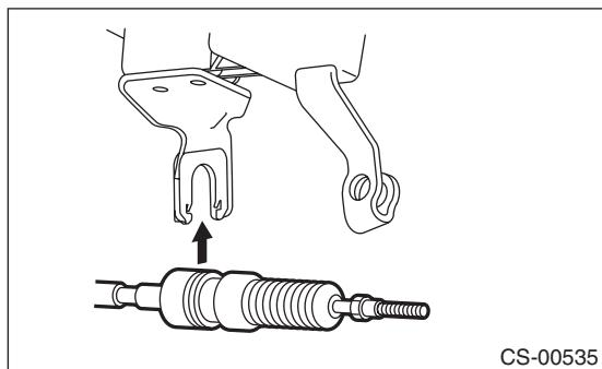
7) Shift the select lever to the "N" range, and then adjust the select cable position. <Ref. to CS-31, ADJUSTMENT, Select Cable.>
