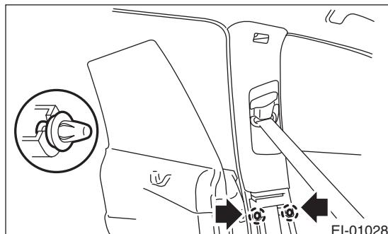
6) Remove the seat belt lower anchor bolt at the center pillar lower port. (Driver's seat)
