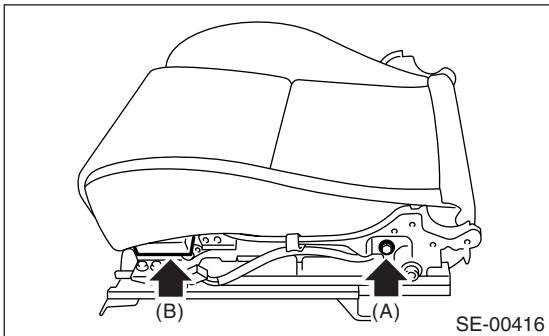
19) Remove the hooks (A), and then remove the seat cushion from seat cushion frame.
