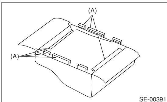
20) Remove the hog rings (A), and then remove the seat cushion cover from seat cushion pad.
