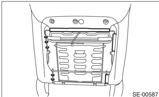
11) Remove the headrest lock bushing.
