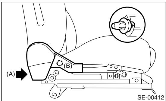
7) Remove the two bolts from the reclining hinge on each left and right side.
