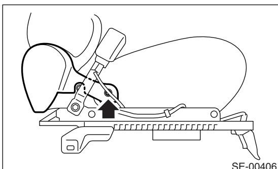
6) Remove the TORX® bolt, and then remove the inner seat belt assembly.
