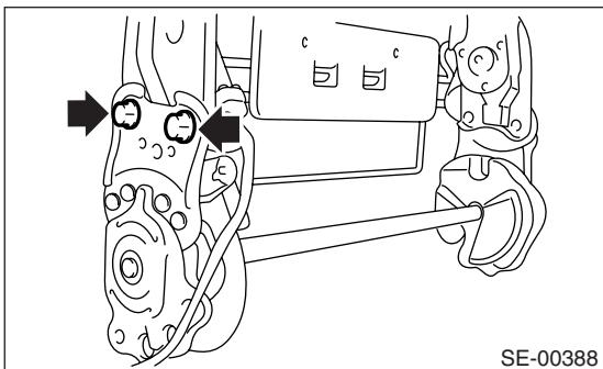
17) Remove the hog rings (A) on the surface side of backrest, and then remove the backrest cover from backrest.
