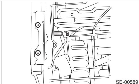
16) Remove the two bolts on each left and right side, and then remove the reclining motor assembly.
