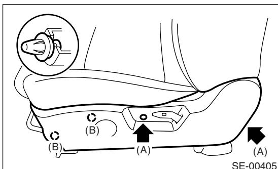
5) Loosen the screws to detach the seat side cover inside.
