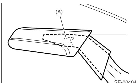
4) Remove screws (A) and clips (B), and then detach the seat side cover outside.
