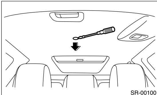
4) Insert the hexagon wrench securely until it touches the motor shaft end.
