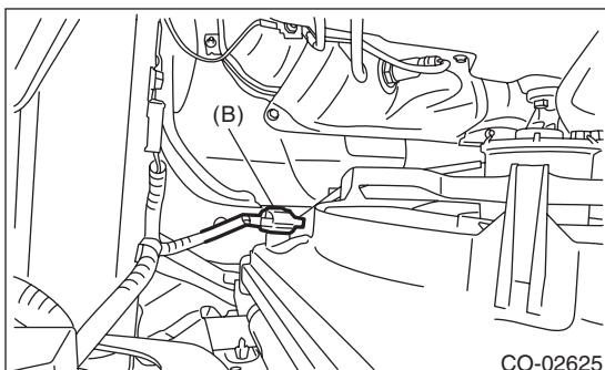
11) Disconnect the radiator inlet hoses from the engine.
