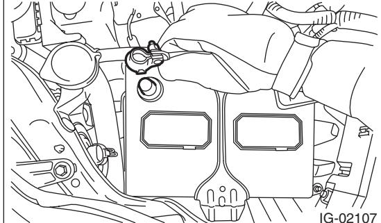
15) Fill engine coolant. <Ref. to CO(H4SO)-13, FILLING OF ENGINE COOLANT, REPLACEMENT, Engine Coolant.>
