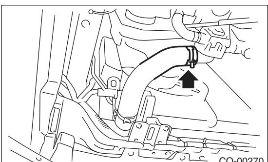
6) Disconnect the CVTF cooler hoses from CVTF pipes. (CVT model)
