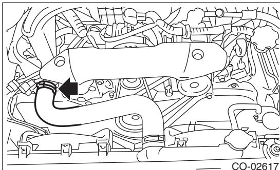
6) Connect the connectors of radiator main fan motor connector (A) and sub fan motor connector (B).
