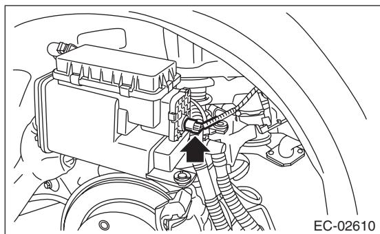
4) Secure the rear wiring harness with clip.
