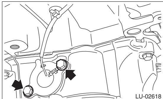
2) Hold the oil level switch harness with the clip.
