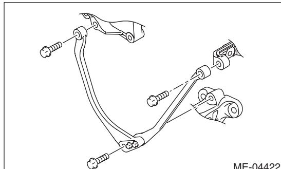
10) Remove the bolt and nut which secure engine mounting to the cradle.
