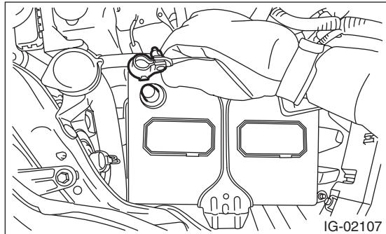
3) Remove the radiator main fan motor assembly and radiator sub fan motor assembly. <Ref. to CO(H4SO)-23, REMOVAL, Radiator Main Fan and Fan Motor.> <Ref. to CO(H4SO)-24, REMOVAL, Radiator Sub Fan and Fan Motor.>
