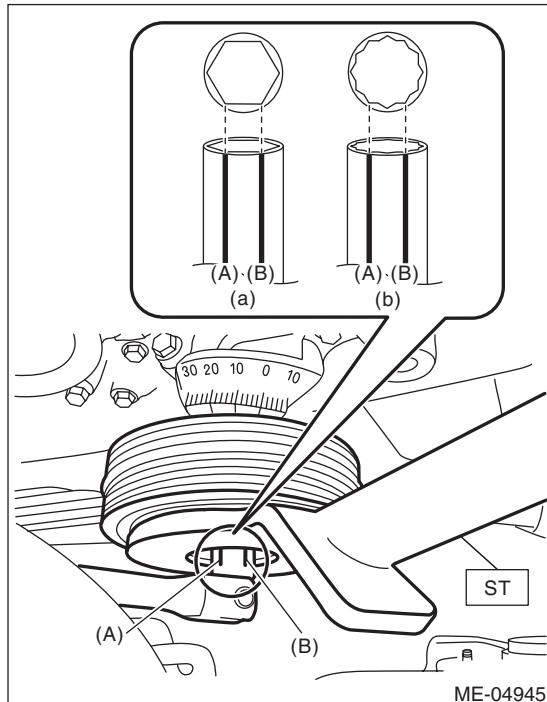
(a) When using 6-point socket
