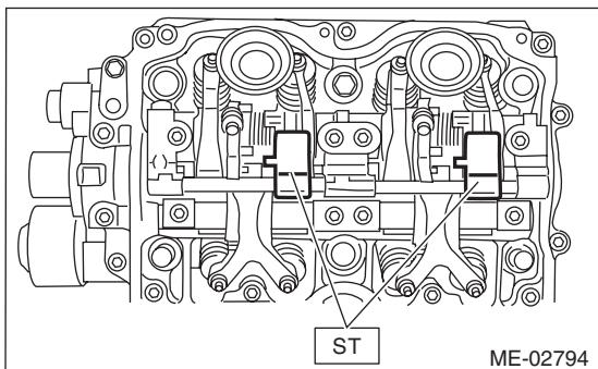
(2) Tighten the bolts (a) through (h) to specified torque.
