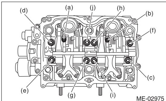
(3) Remove the valve rocker assembly.
