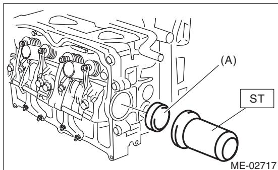
5) Install the camshaft position sensor support. (LH side only)
