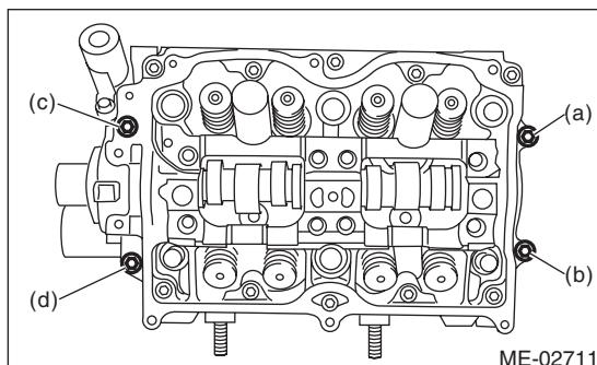
(3) Install the valve rocker assembly. <Ref. to ME(H4SO)-54, INSTALLATION, Valve Rocker Assembly.>
