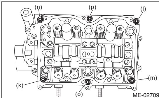
(4) Remove the camshaft cap.
