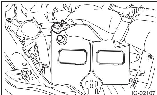
2) Remove the air intake boot assembly. <Ref. to IN(H4SO)-8, REMOVAL, Air Intake Boot.>
