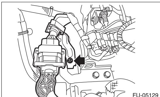
4) Slide the engine harness connector in the direction of the arrow and remove it from the rear engine hanger.
