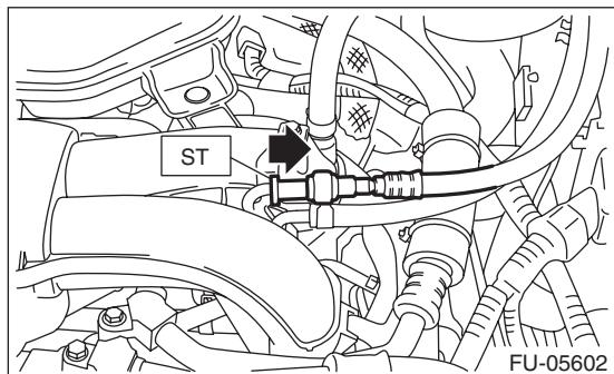
(2) Connect the fuel pressure gauge with ST2 and ST3.
