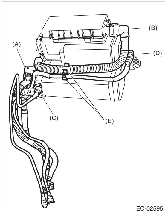
3) Install the canister to the vehicle.
