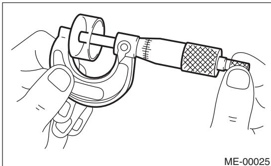
5) Select a valve lifter of suitable thickness using the measured valve clearance and valve lifter thickness, and install it.
