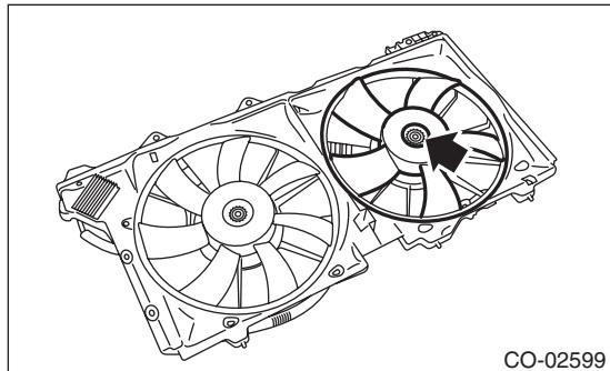
3) Remove the radiator main fan motor.
