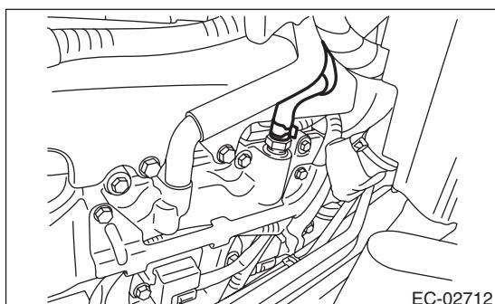
4) Remove the PCV valve from rocker cover.
