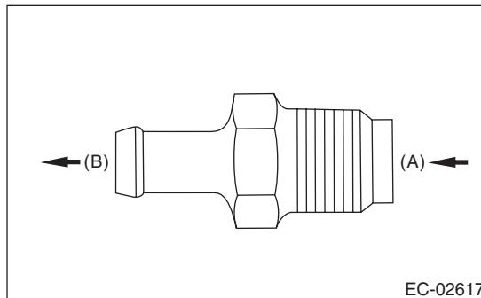
3) Check that air does not come out from (B) when air is blown into (A).
