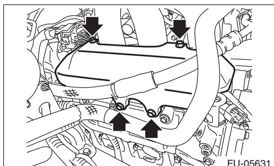
7) Disconnect the connector from fuel injector.
