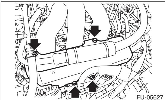
8) Disconnect the connector from fuel injector.
