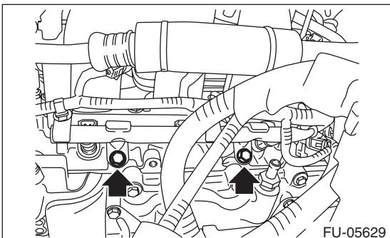
10) Remove the fuel injector while lifting up the fuel injector pipe.
