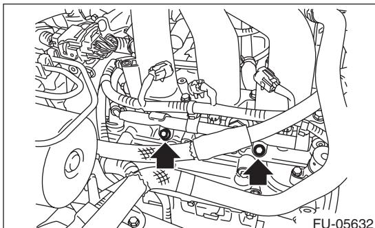
9) Remove the fuel injector while lifting up the fuel injector pipe.
