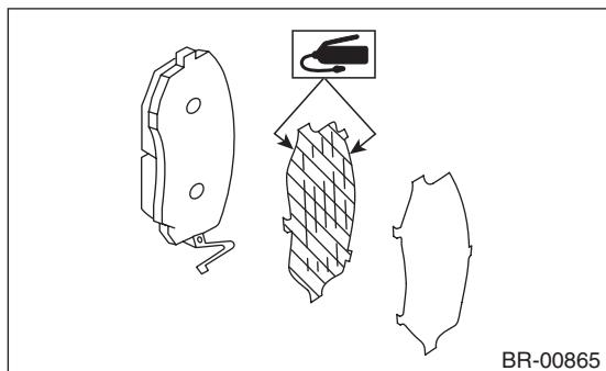
4) Install the brake pad to the support.
