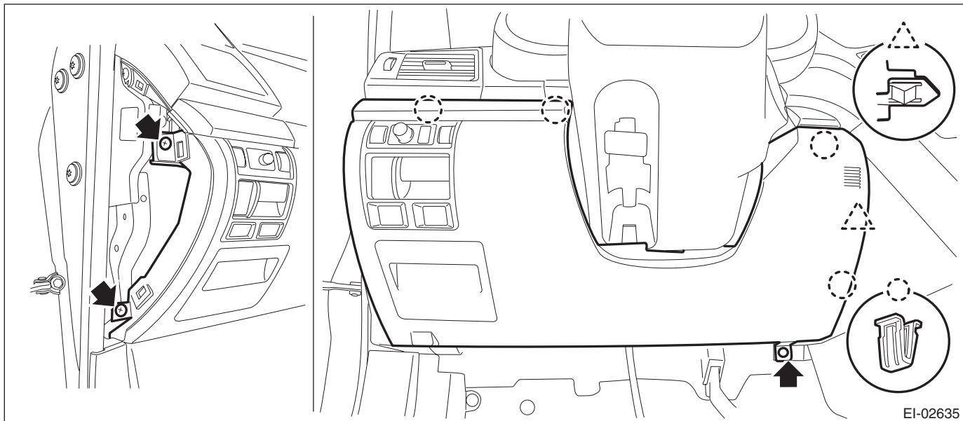
3) Remove the screws and remove the parking brake switch.
