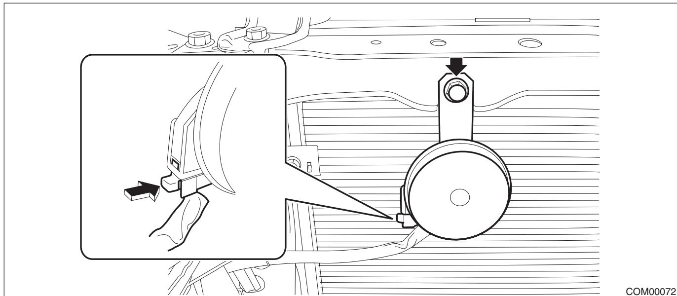
6) Remove the Hi pitch side horn.
