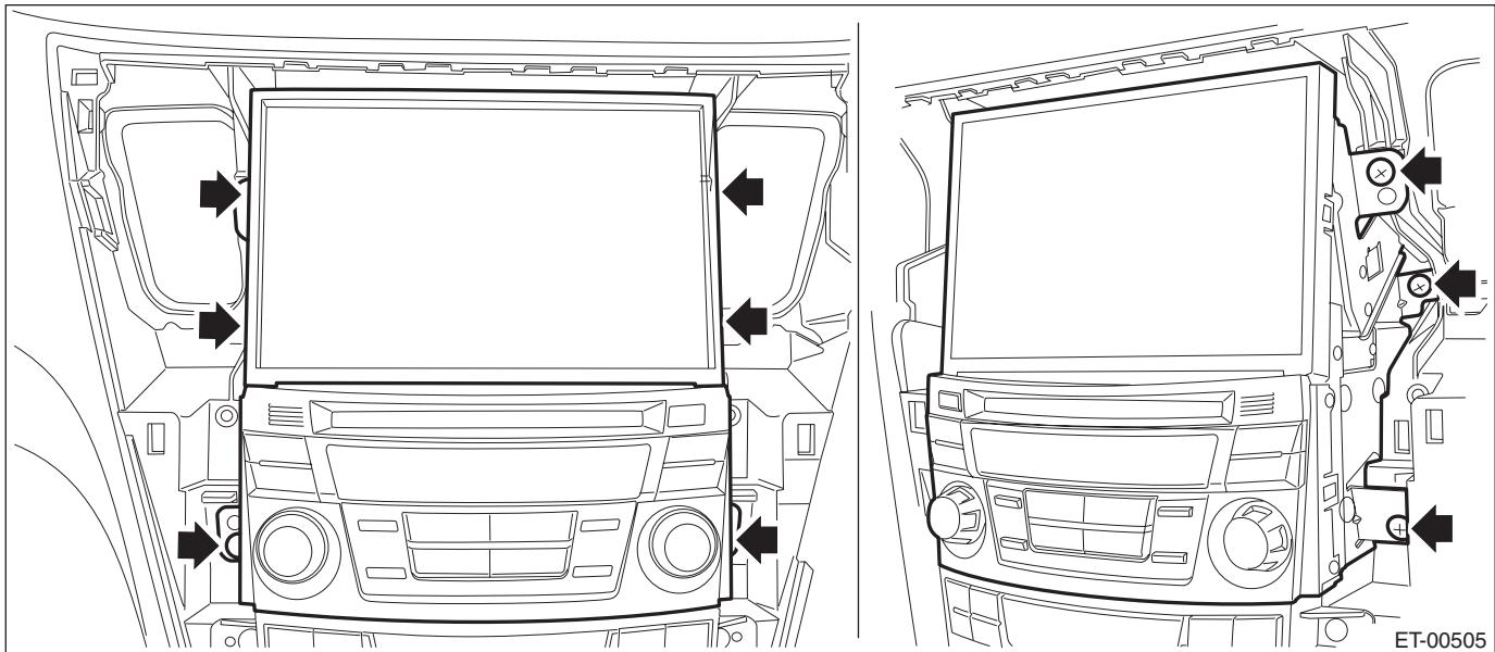
5) Remove the control panel assembly.
