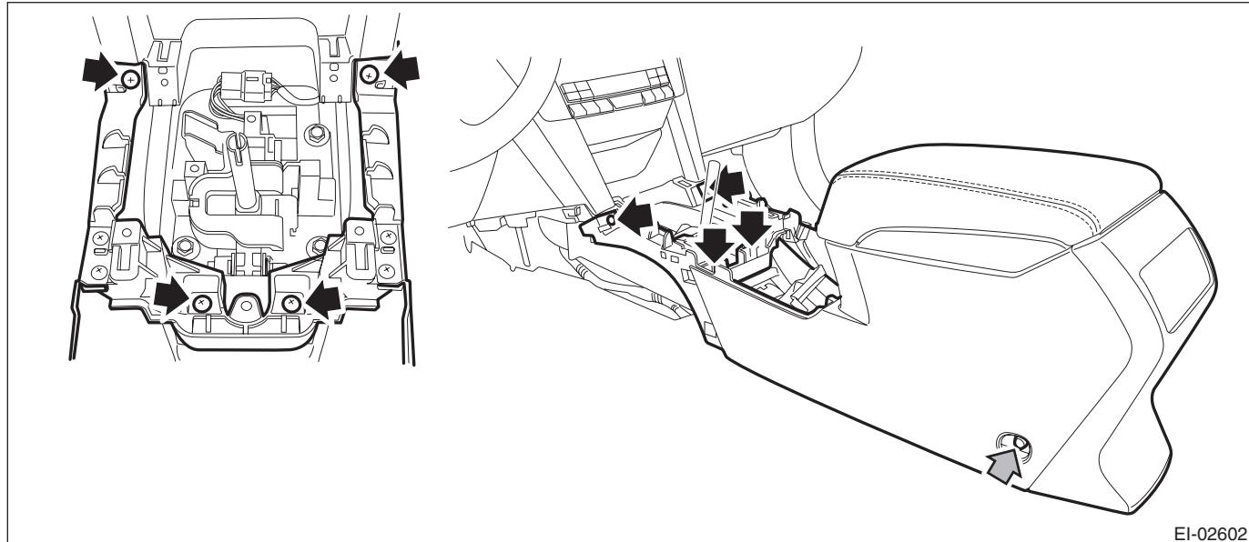
4) Remove the front accessory power supply socket.
