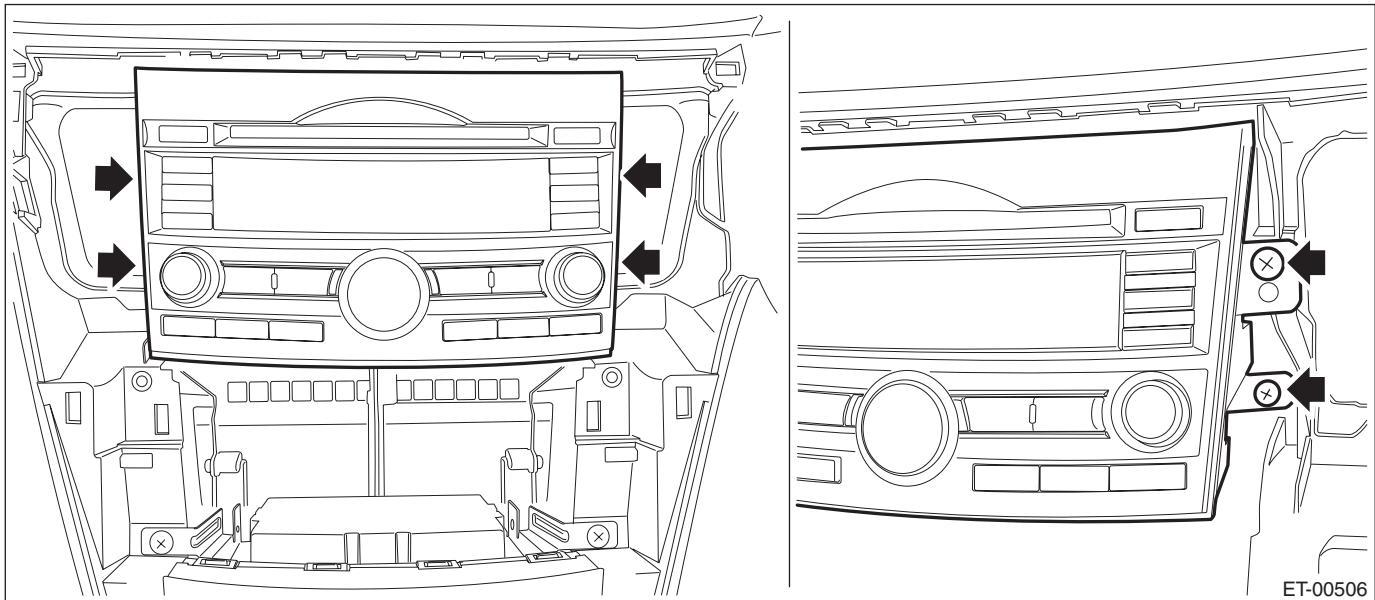
6) Remove the navigation assembly. (model with navigation)
