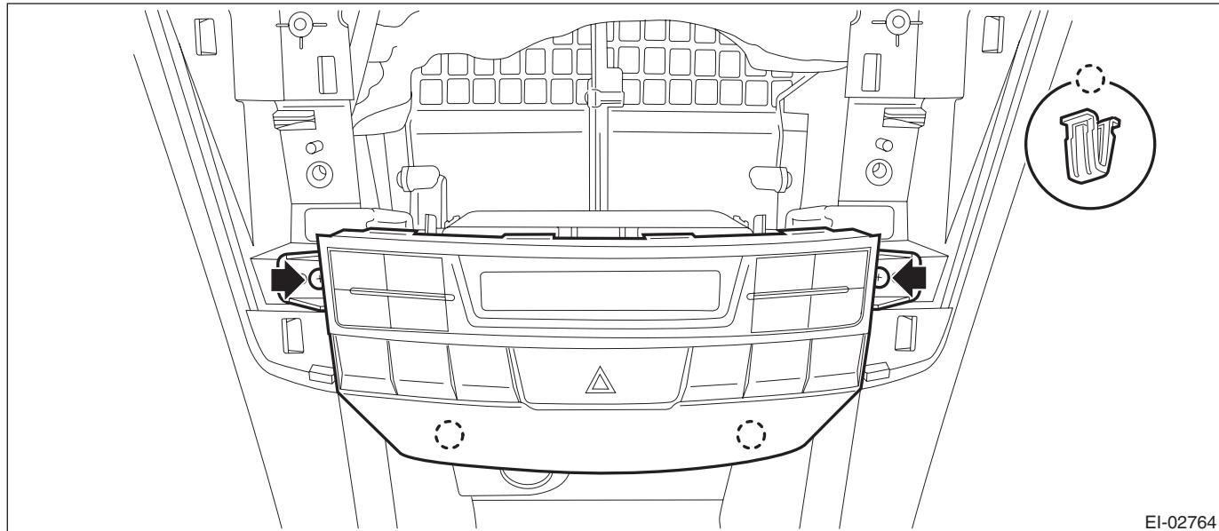
(2) Remove the screws, and pull out the tuner unit.
