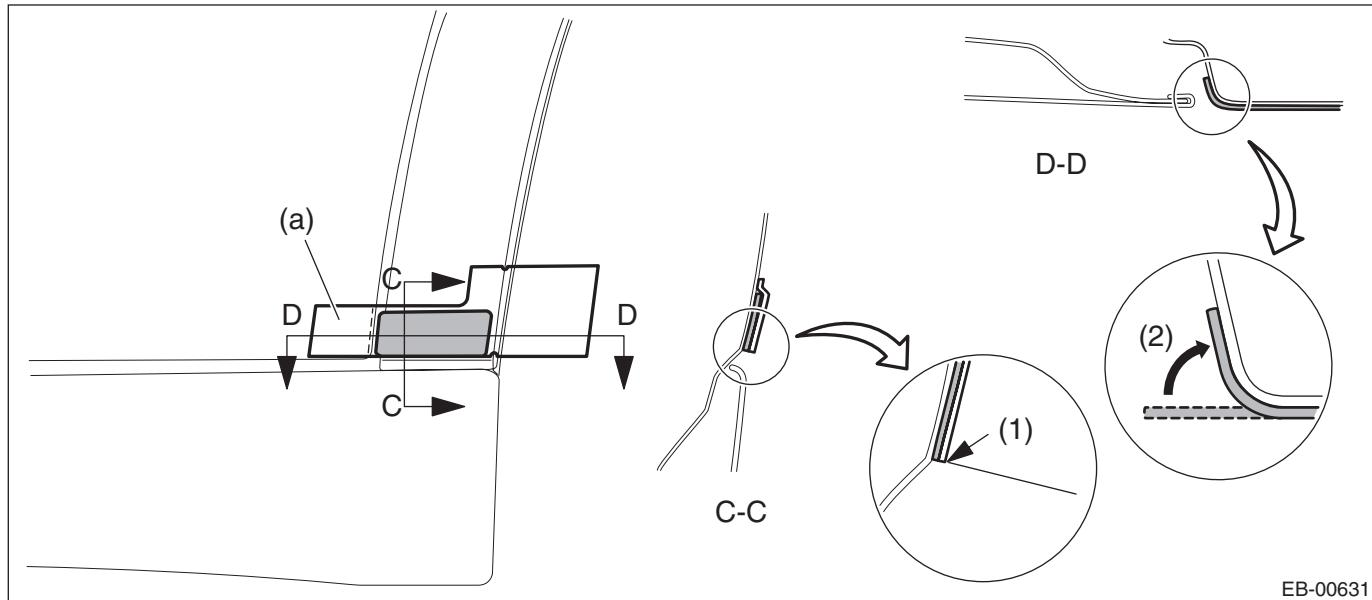
(1) Align the application sheet to the end of rounded corner.
