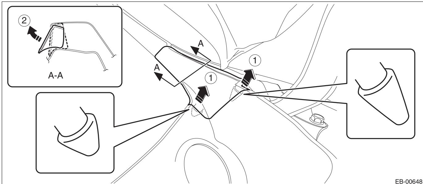
3) Remove the front fender panel. <Ref. to EB-16, REMOVAL, Front Fender.>
