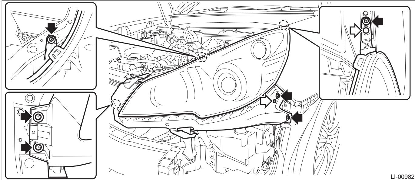
b) Disconnect the connector and remove the headlight assembly.
