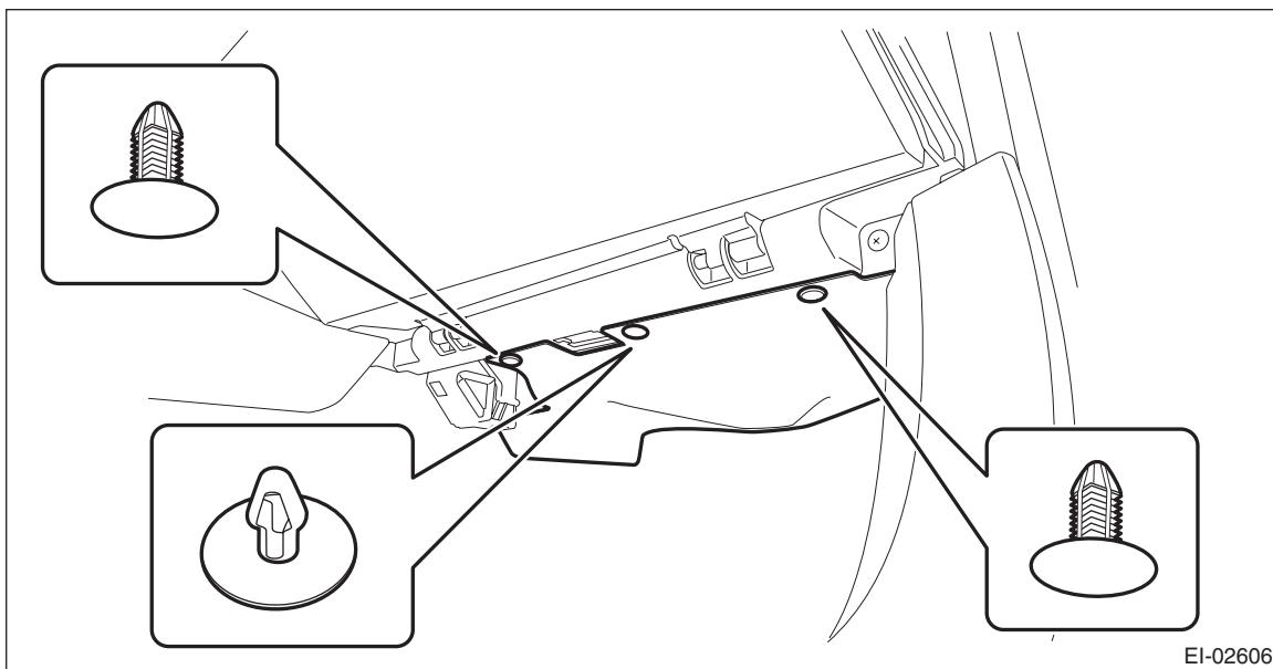
(2) Release the clips and claws, and remove the ornament panel assembly P.
