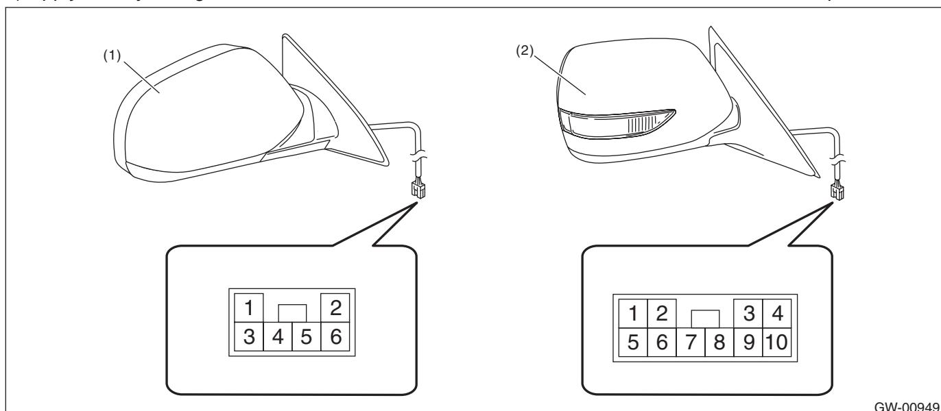
(1) Model without electric retractable mirror
