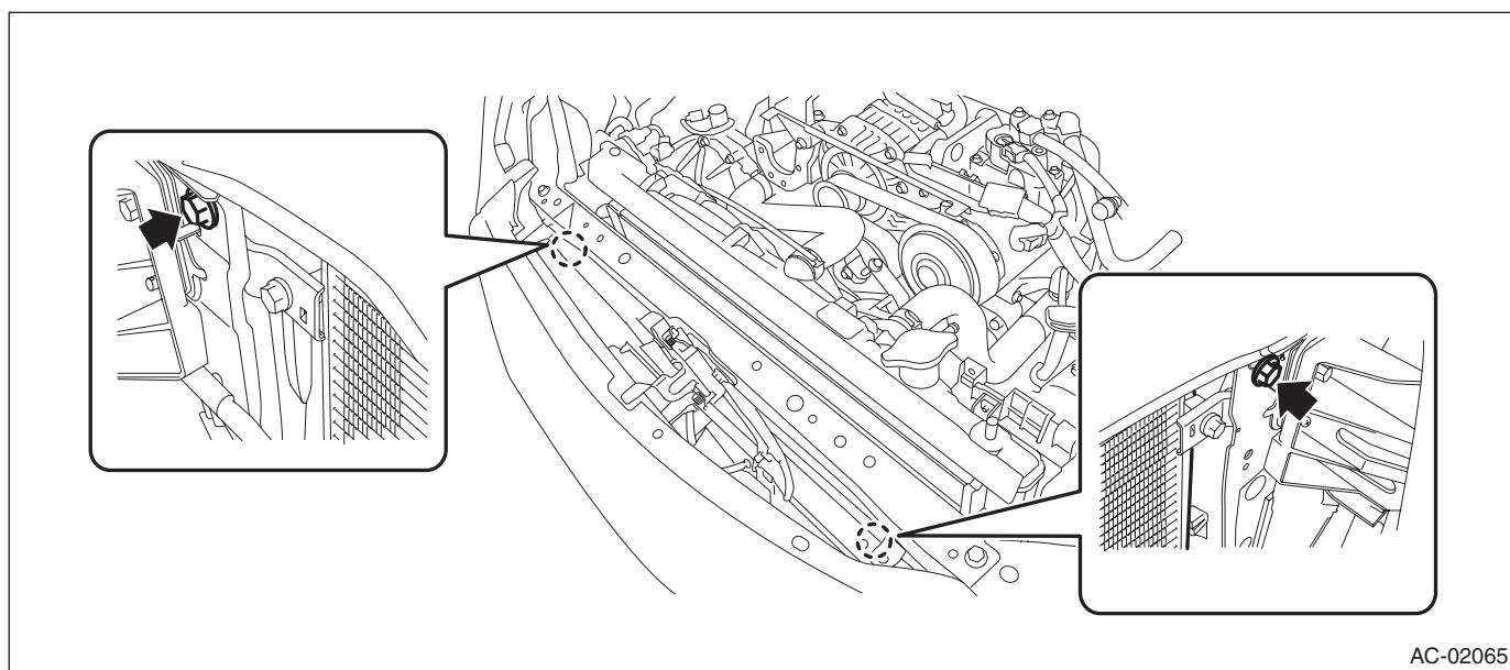
(2) By lifting the condenser, pull it out through the space between the radiator and the radiator panel.
