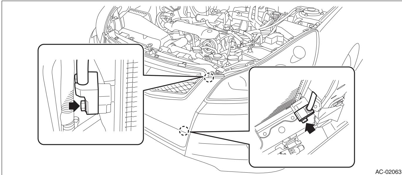
5) Remove the bolts and remove the radiator upper bracket.
