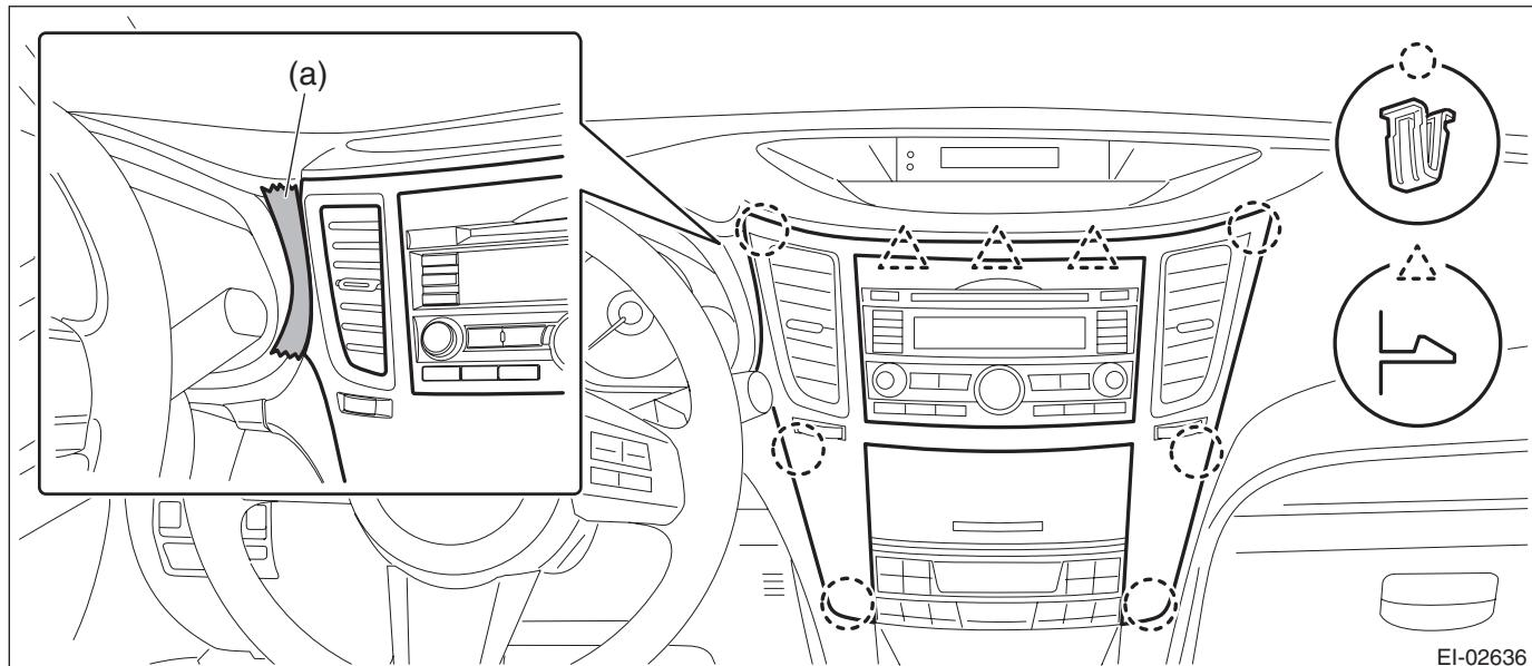
(2) Insert a finger into the air vent grille and release the left and right clips at the top of the center panel.
