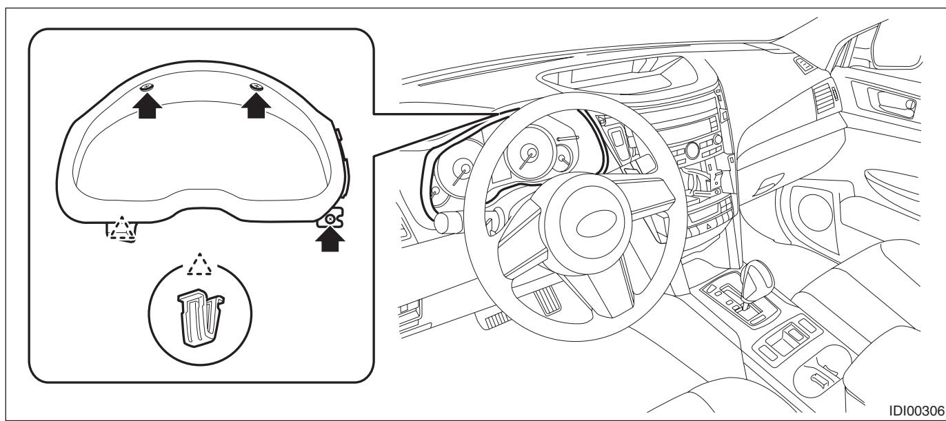
6) Remove the combination meter assembly.
