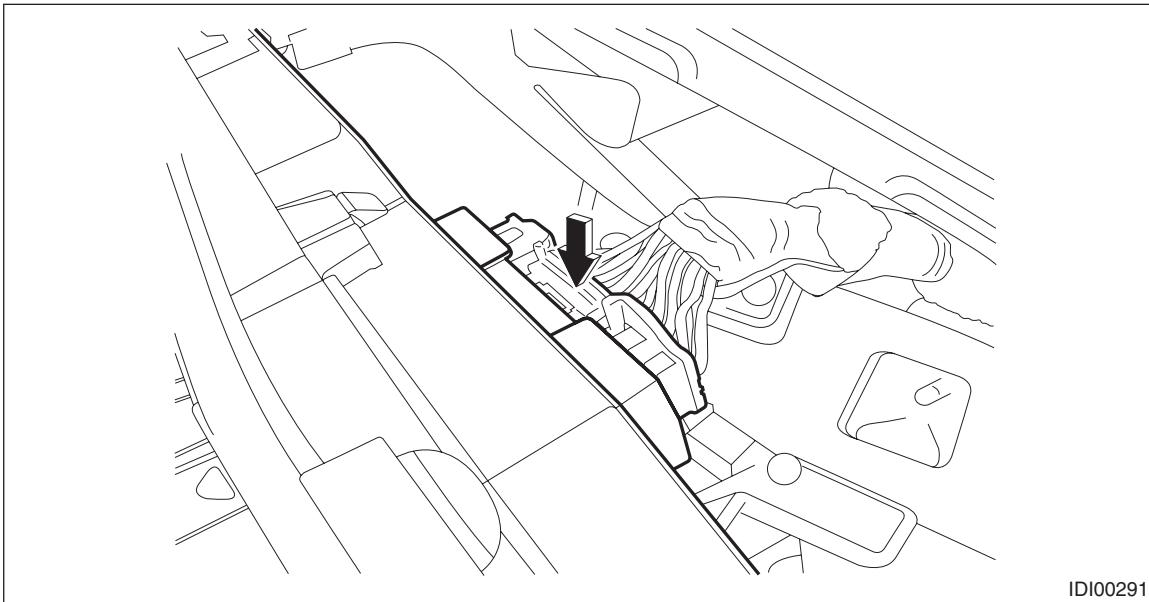
(4) Remove the combination meter assembly as shown in the figure.
