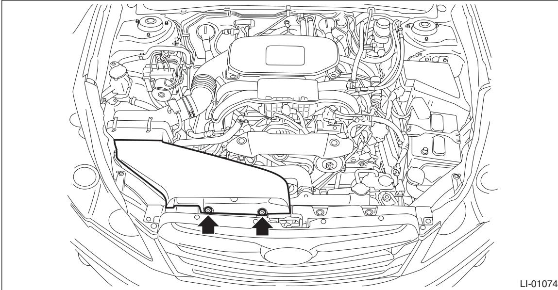
3) Turn the steering wheel in the opposite direction to the headlight to be removed. Then remove the clips and turn over the mud guard.
