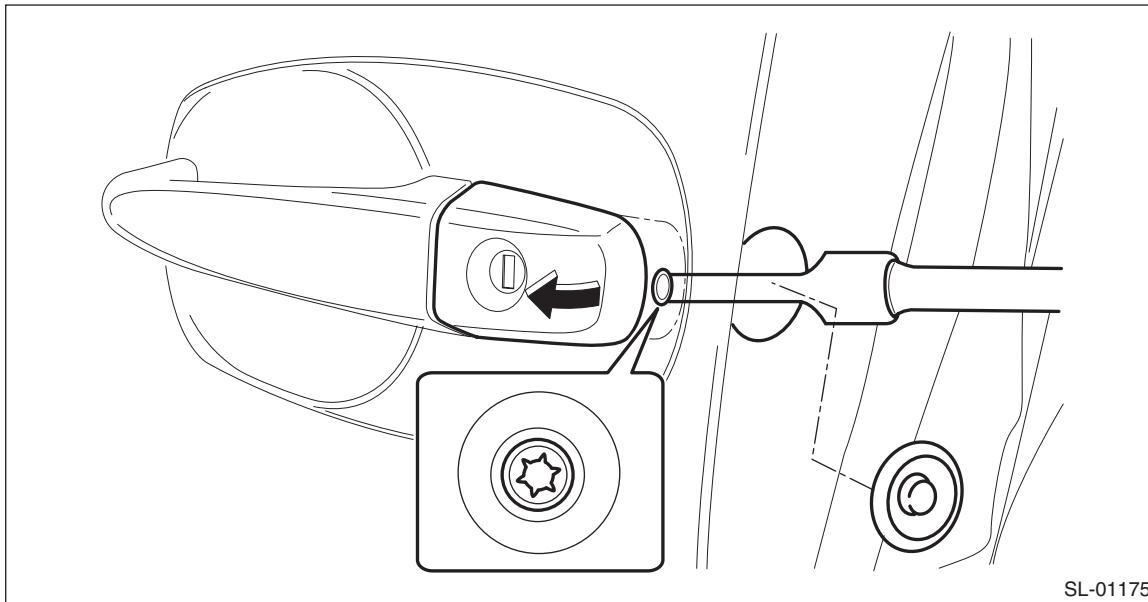
6) Move the front outer handle to the rear and remove the front outer handle.
