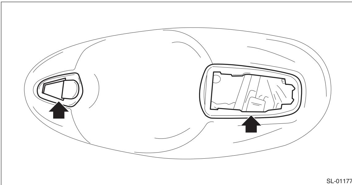
(2) Loosen the TORX® bolt and remove the frame assembly from the door panel.
