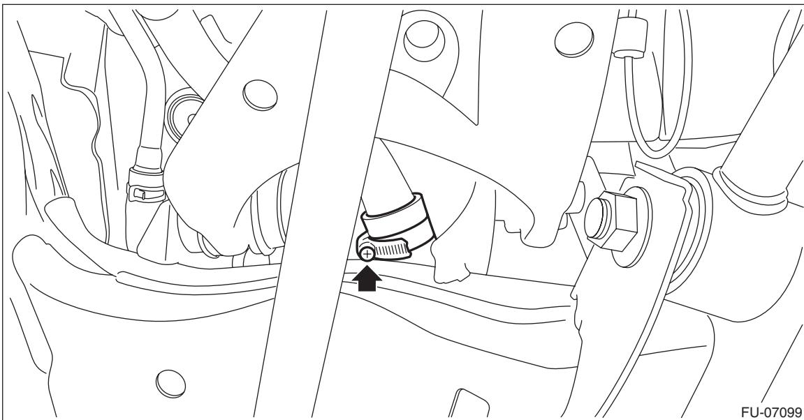
6) Set the container under the vehicle and insert the gasoline proof hose ( $\varnothing 10$  or less) into the fuel filler hose to drain the fuel.
