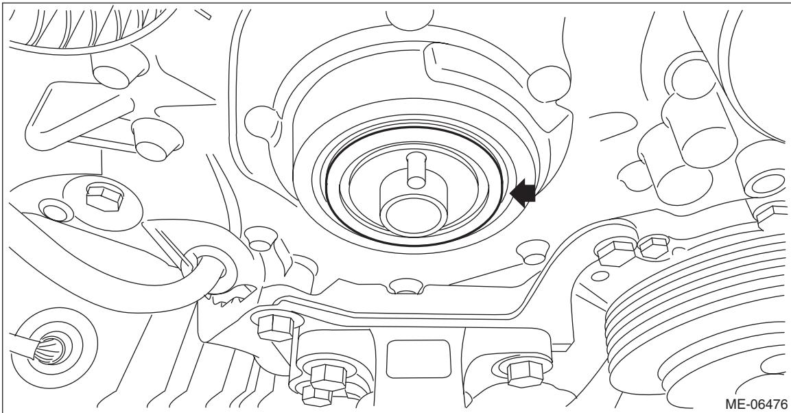
4) Apply engine oil to the crank pulley bolt seat and thread.
