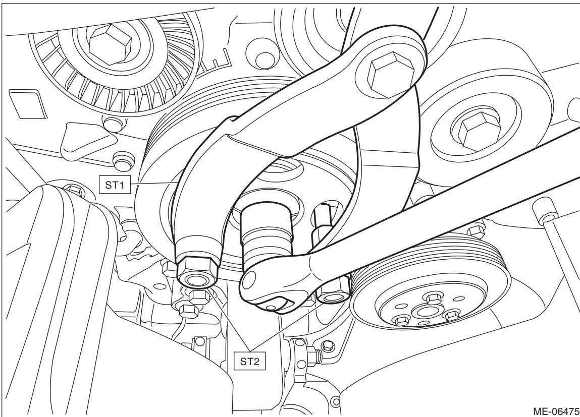
3) Remove the crank pulley and remove the crank pulley boss.
