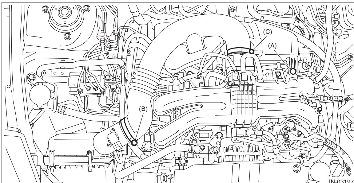
(3) Remove the air intake boot from the throttle body, and move it to the left side wheel apron.
