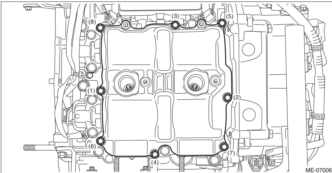
5) Install the intake manifold protector RH.
