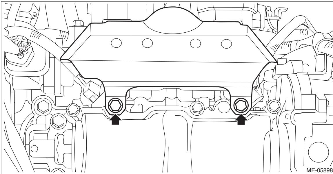
6) Install the #1 ignition coil and the #3 ignition coil. <Ref. to IG(H4DO)-9, INSTALLATION, Ignition Coil.>
