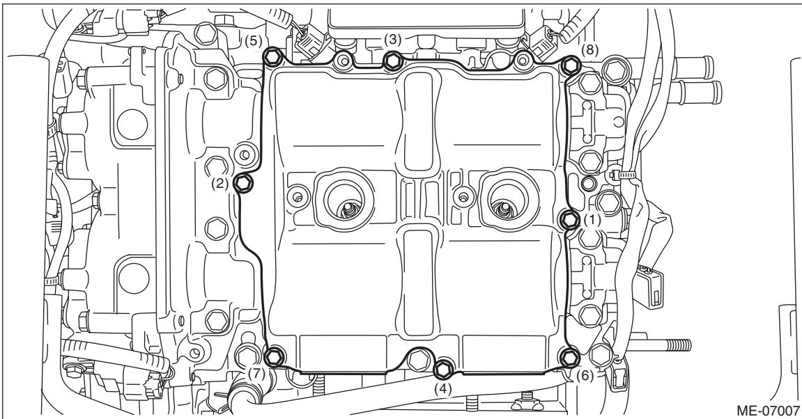
6) Install the intake manifold protector LH.
