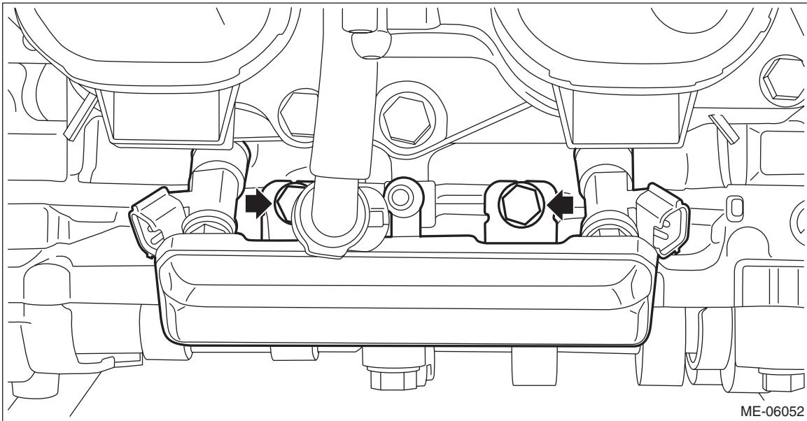
10) Insert the steel rods into ST, and set the engine so that the camshaft LH is facing up.
