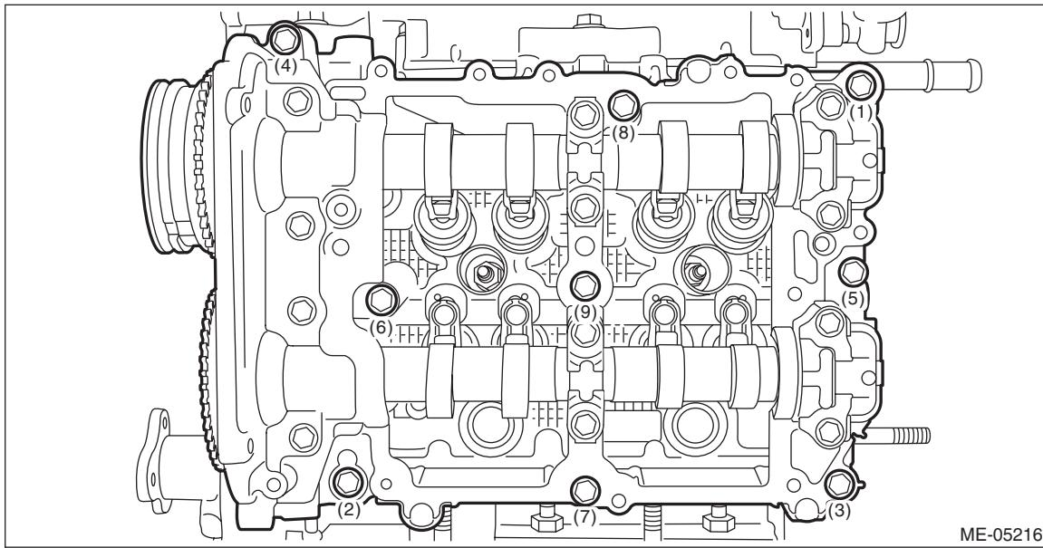
12) Remove the O-ring and the roller rocker arm from cylinder head LH.
