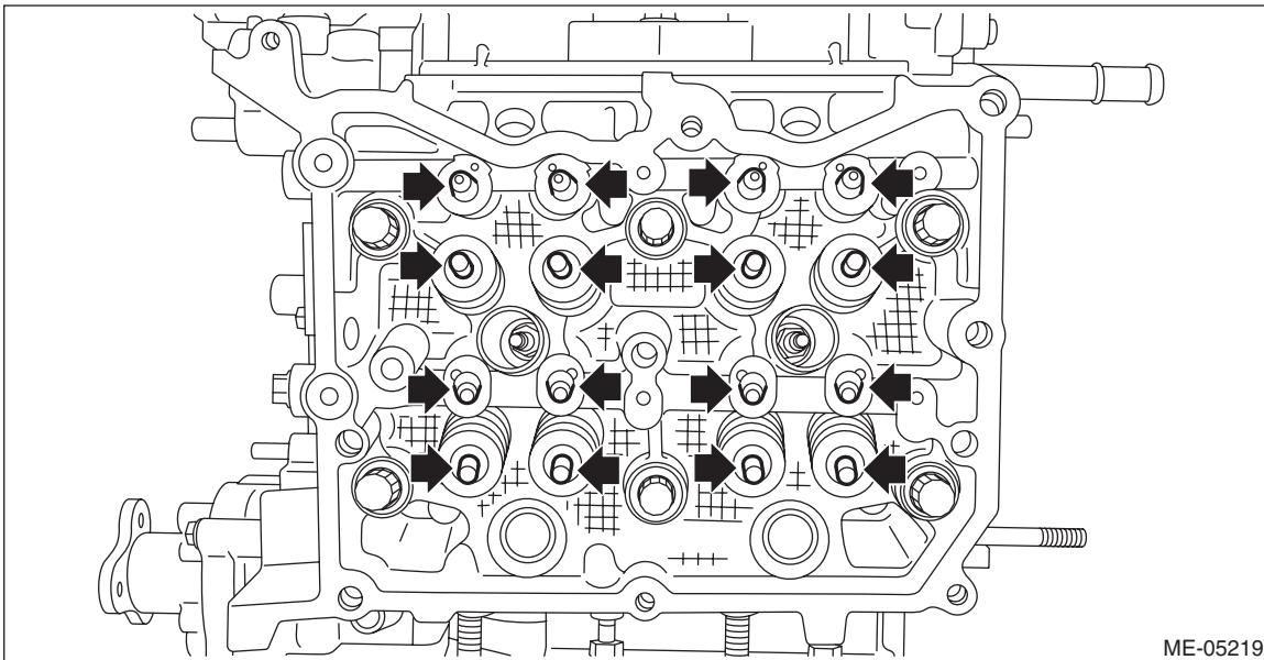
14) Remove the liquid gasket from cam carrier LH and cylinder head LH.
