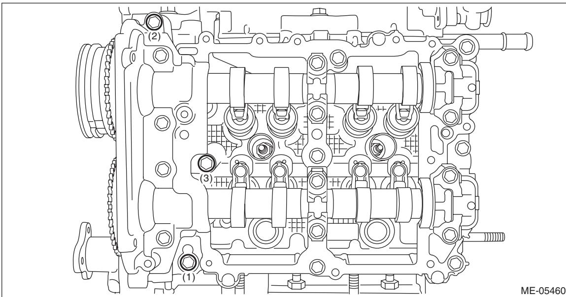
(5) Tighten the bolts (3 places) with a torque of 18 N·m (1.8 kgf-m, 13.3 ft-lb) in numerical order as shown in the figure.
