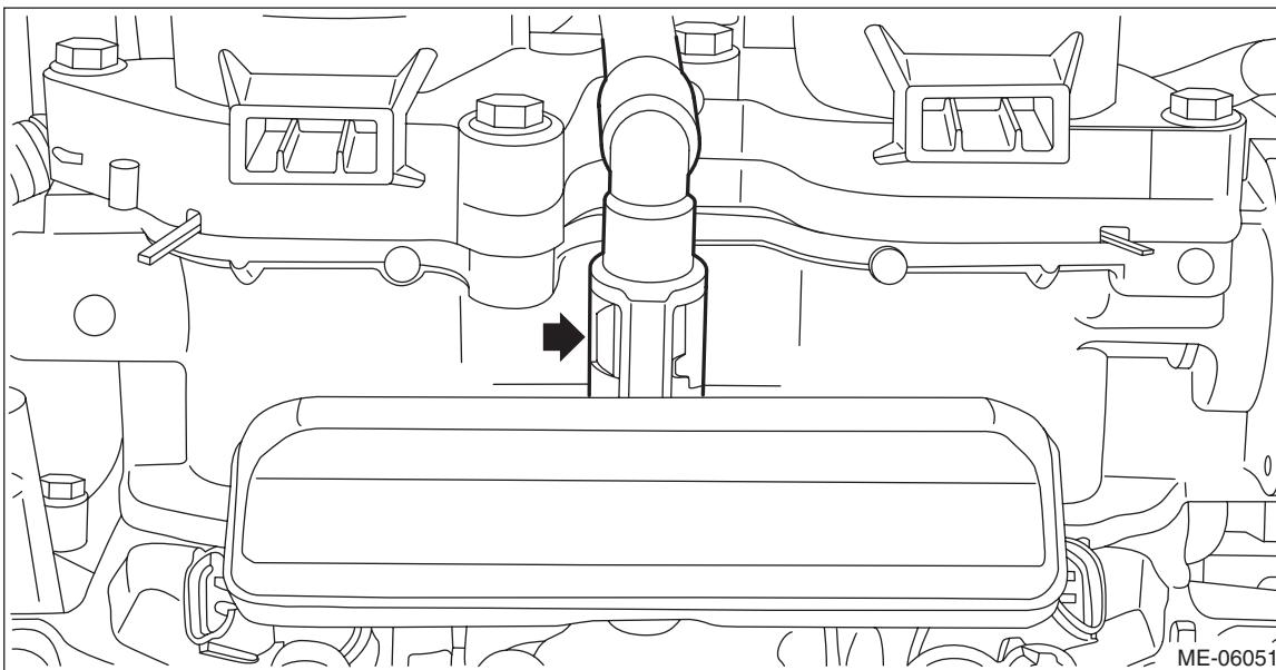
(3) Connect the connectors to the fuel injector LH.
