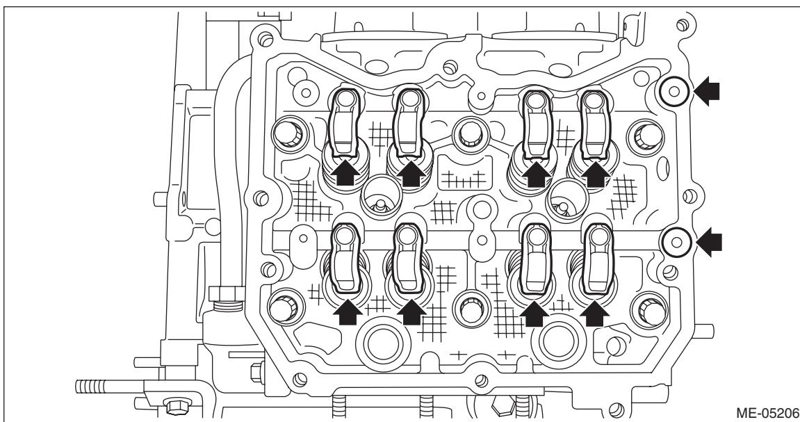
11) Remove the valve shim and the roller rocker arm pivot from cylinder head RH.
