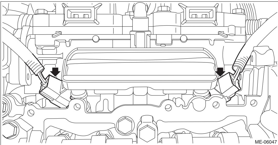
11) Secure the engine harness to the cam carrier RH with a clip.
