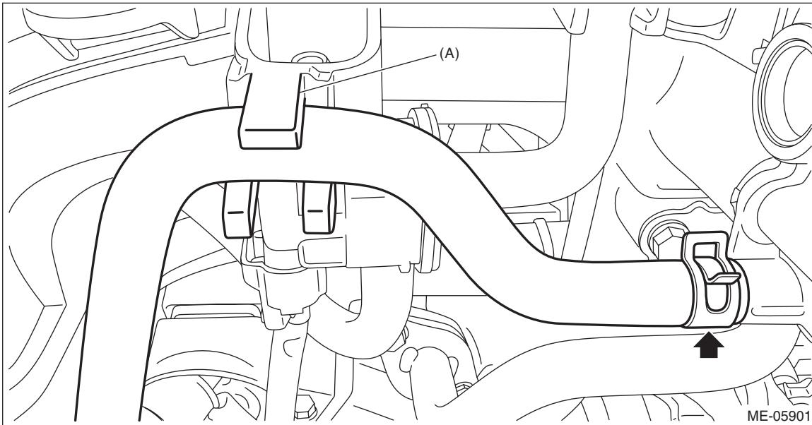
13) Secure the engine harness to the cam carrier LH with a clip.
