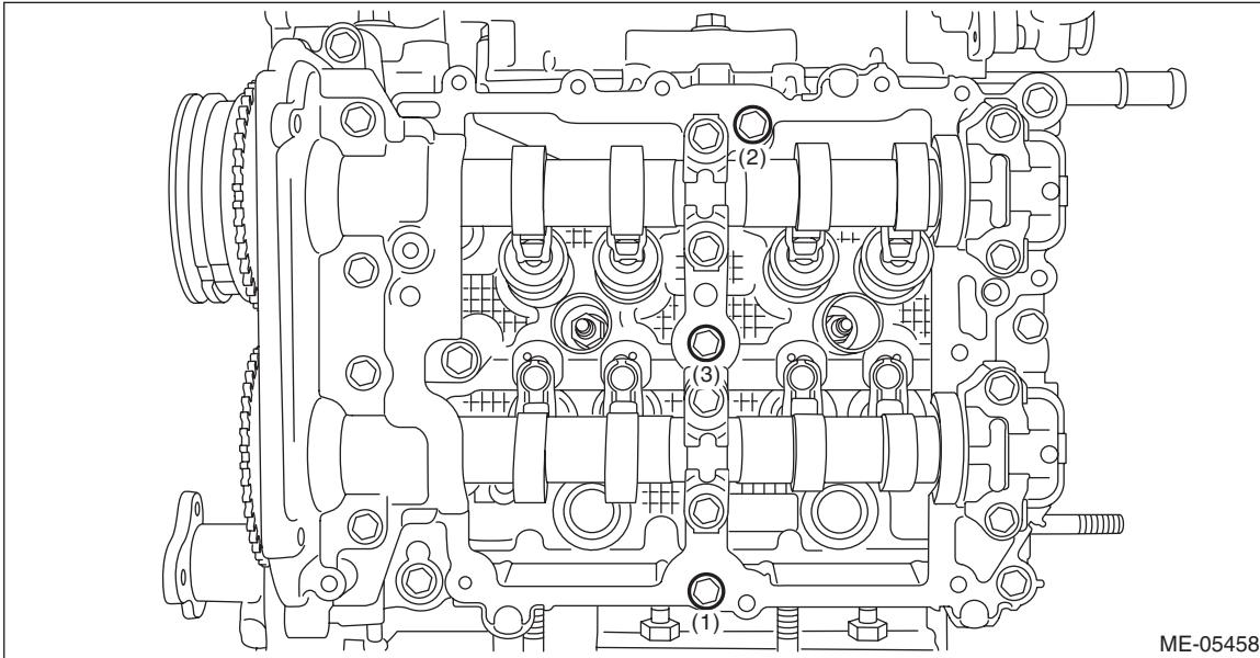
(3) Tighten the bolts (3 places) with a torque of 18 N·m (1.8 kgf-m, 13.3 ft-lb) in numerical order as shown in the figure.
