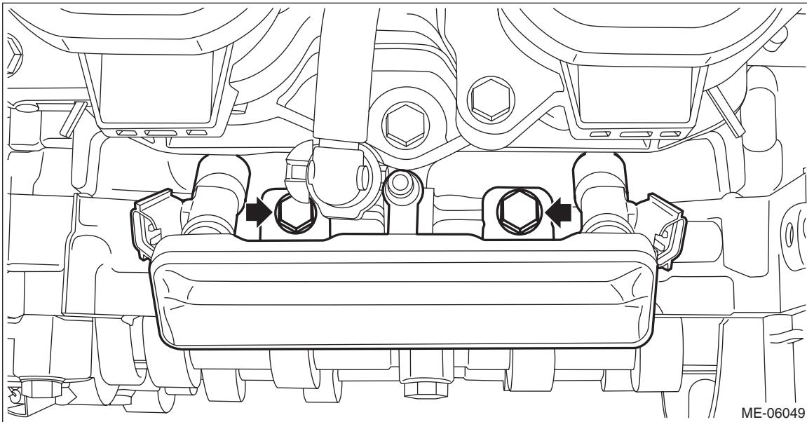
8) Insert the steel rods into ST, and set the engine so that the camshaft RH is facing up.
