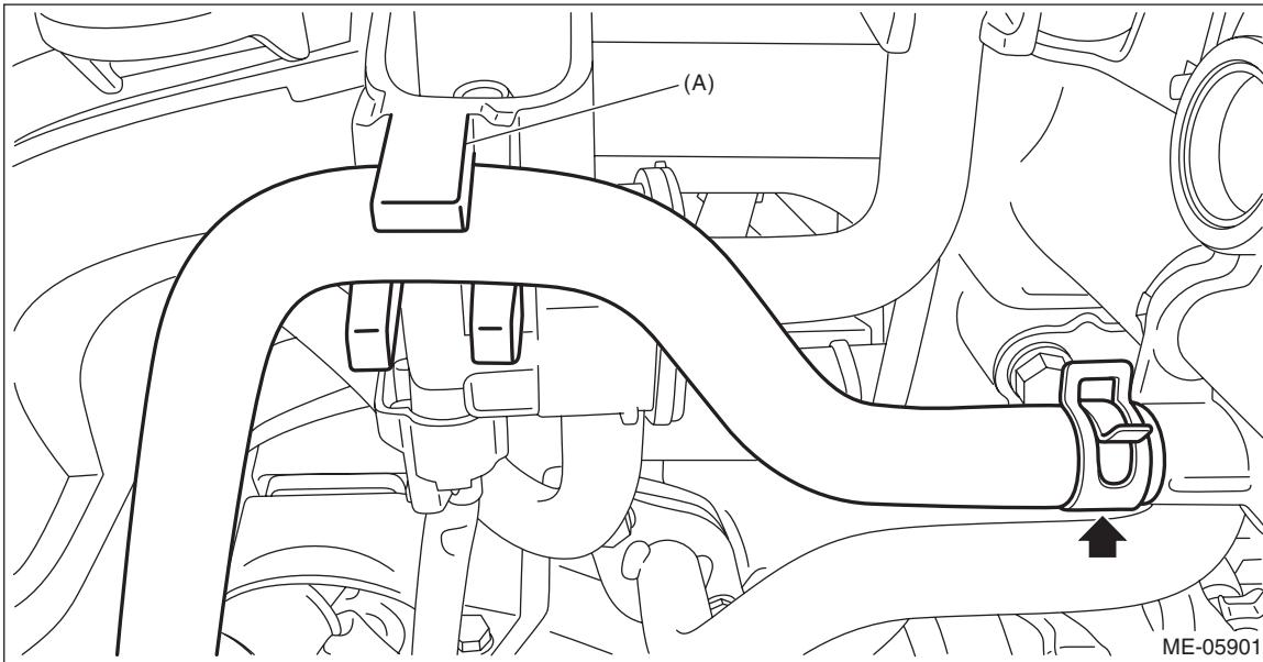
8) Disconnect the water pipe hose from oil pan upper, and remove the water pipe assembly.
