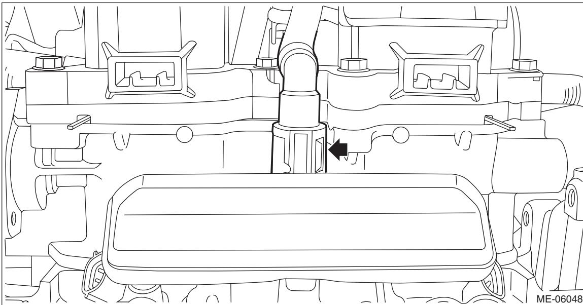
(3) Remove the bolts securing the fuel pipe RH, and remove the fuel pipe RH and the fuel injector RH.
