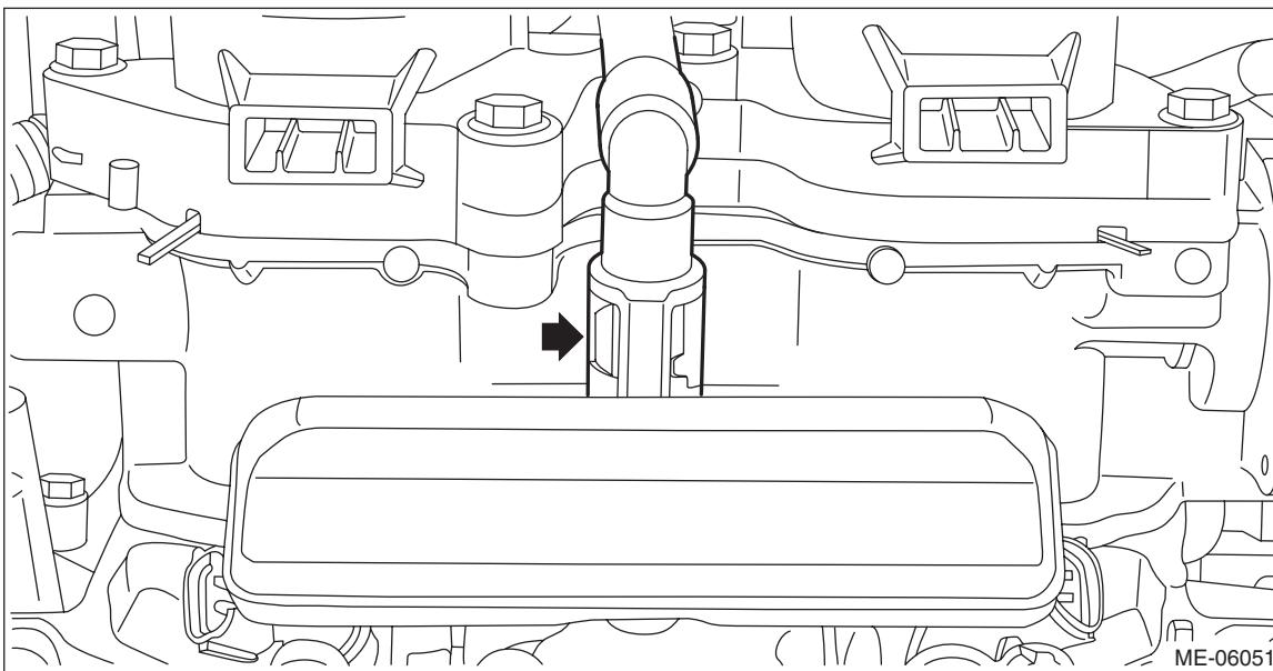
(3) Remove the bolts securing the fuel pipe LH, and remove the fuel pipe LH and the fuel injector LH.
