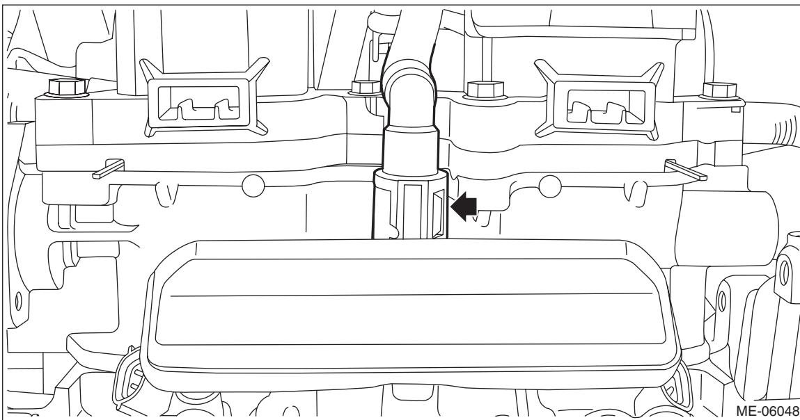
(3) Connect the connectors to the fuel injector RH.
