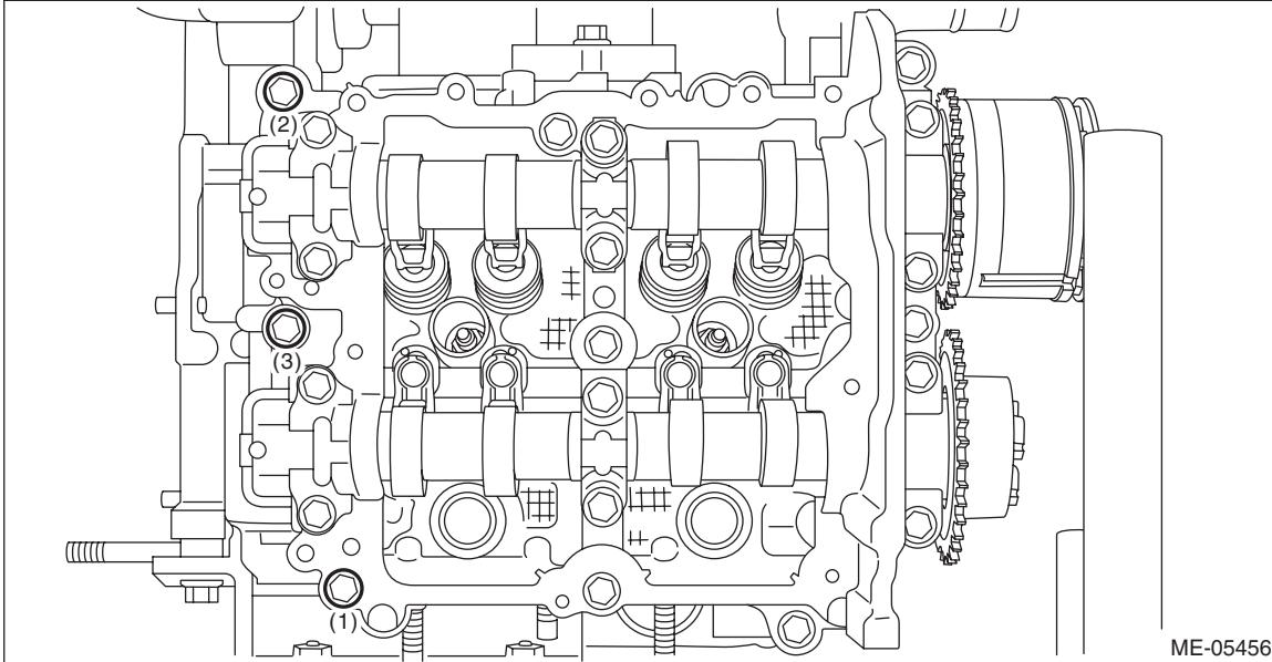
(7) Tighten the bolts (3 places) with a torque of 18 N·m (1.8 kgf-m, 13.3 ft-lb) in numerical order as shown in the figure.
