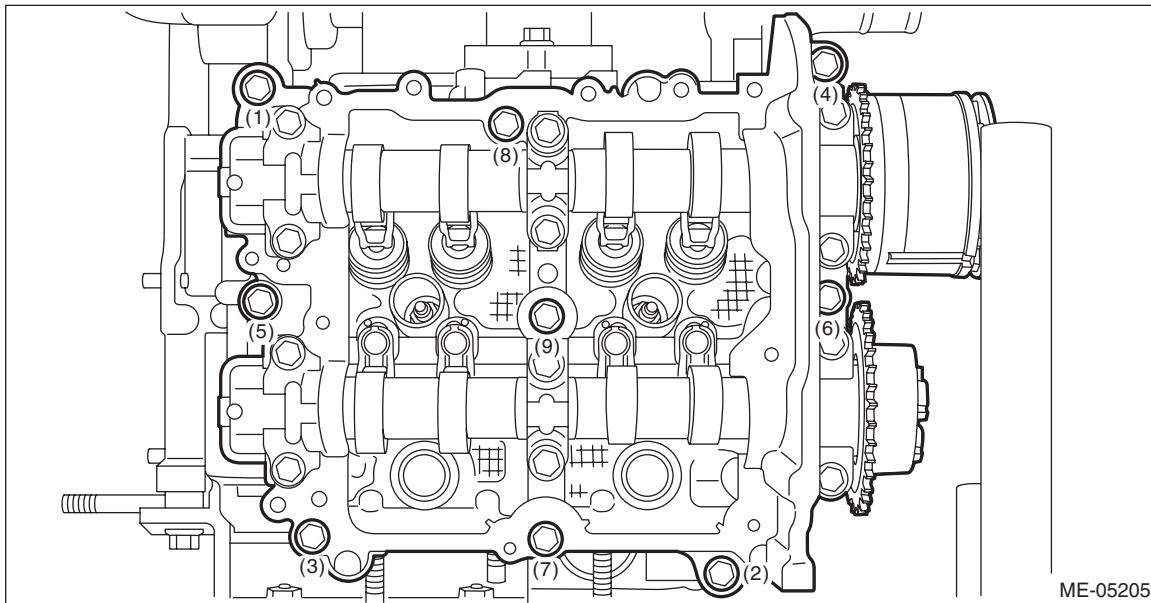
10) Remove the O-ring and the roller rocker arm from cylinder head RH.
