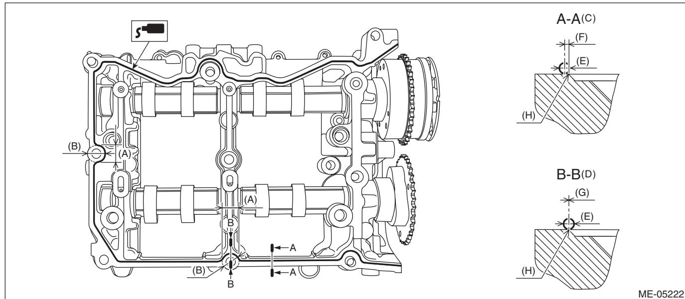
(A) Range A (D) Liquid gasket applying position of mating surfaces of range A (G)  $0 \pm 0.5$  mm ( $0 \pm 0.0197$  in)
