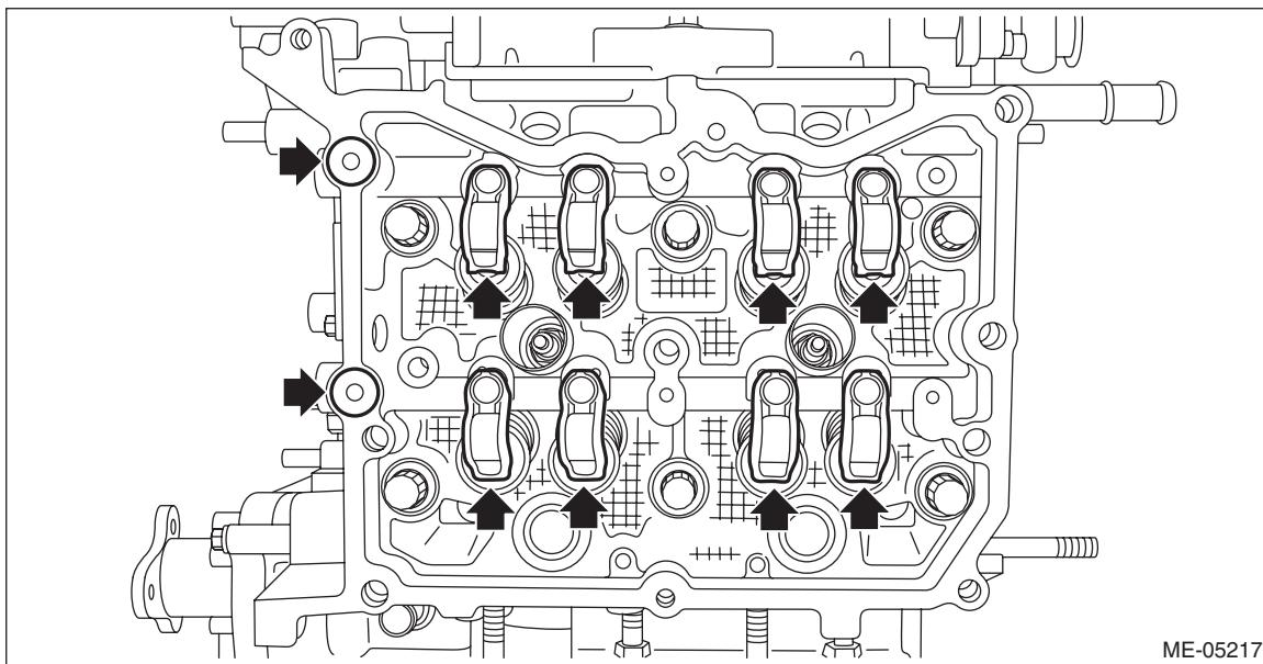
13) Remove the valve shim and the roller rocker arm pivot from cylinder head LH.
