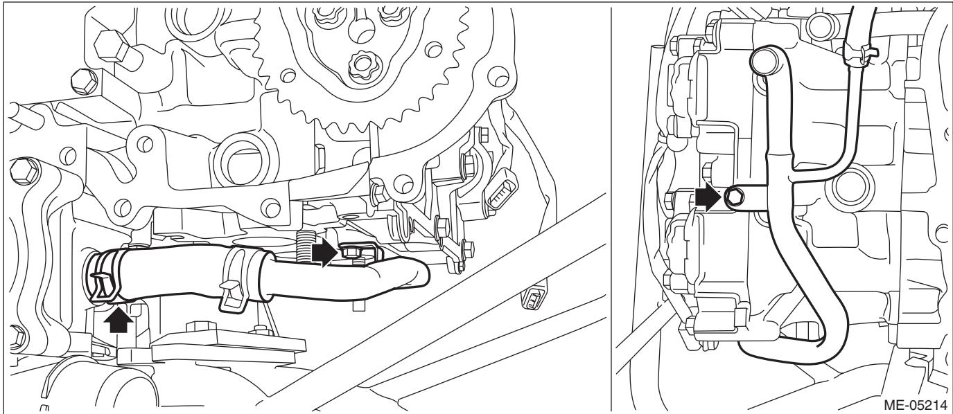
9) Remove the fuel pipe LH and the fuel injector LH.
