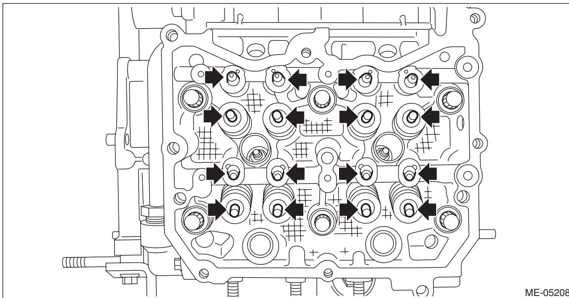
12) Remove the liquid gasket from cam carrier RH and cylinder head RH.
