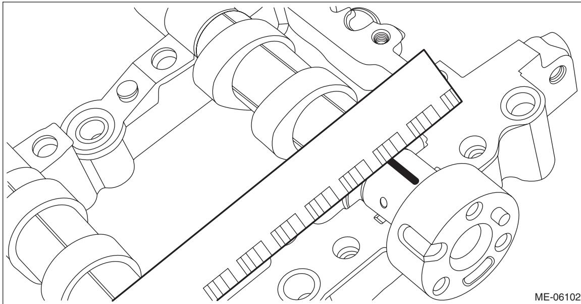
(8) Completely remove the plastigauge.
