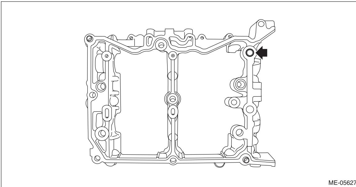
4) Remove the liquid gasket from cam carrier LH and front camshaft cap LH, intake rear camshaft cap LH and exhaust rear camshaft cap LH.
