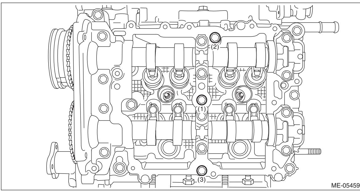
(4) Loosen the bolts (3 places) by  $180^{\circ}$  in numerical order as shown in the figure.
