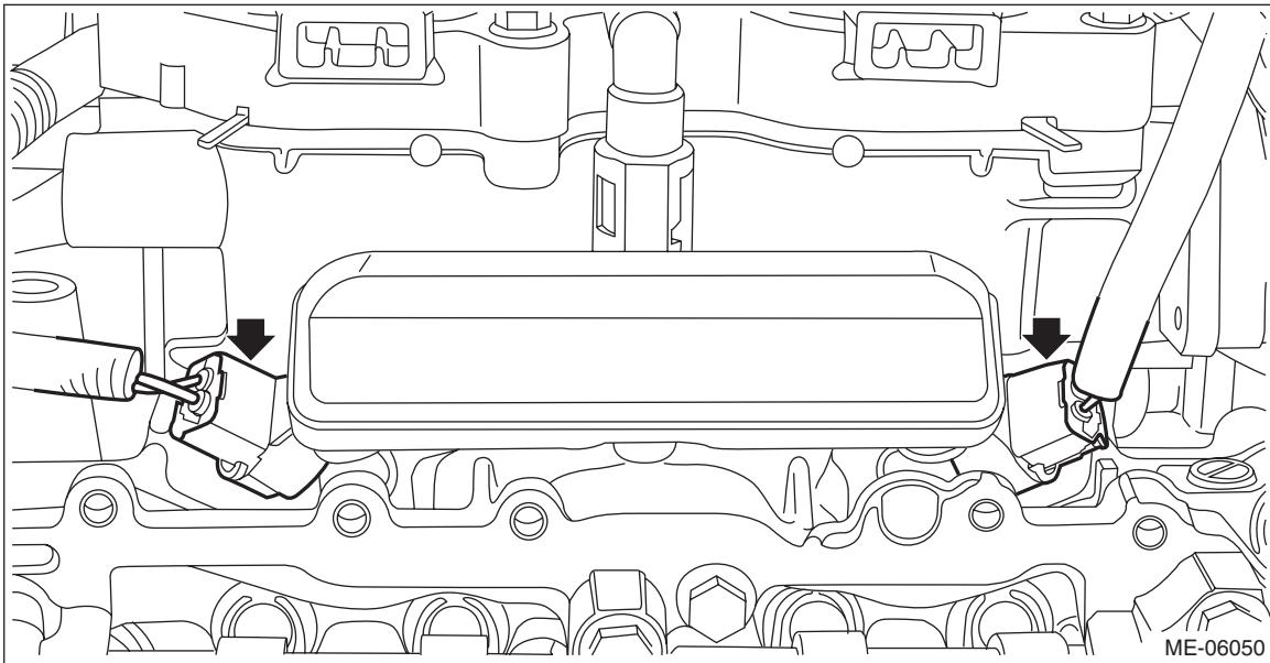
11) Connect the water pipe hose to oil pan upper, and install the water pipe assembly.
