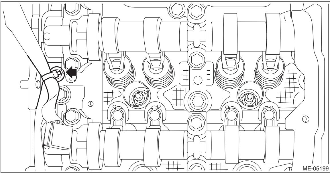
12) Install the rocker cover RH. <Ref. to ME(H4DO)-145, ROCKER COVER RH, INSTALLATION, Rocker Cover.>
