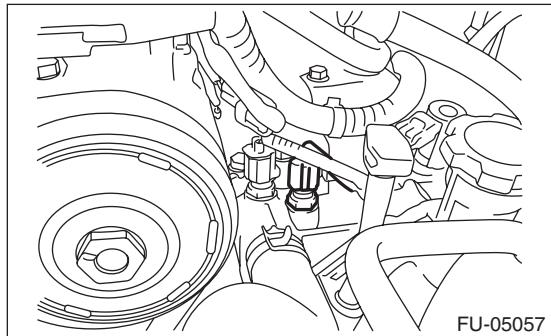
4) Remove the oil temperature sensor.
