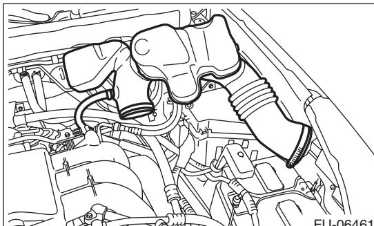
9) Remove the air cleaner case. <Ref. to IN(H6DO)-5, REMOVAL, Air Cleaner Case.>
