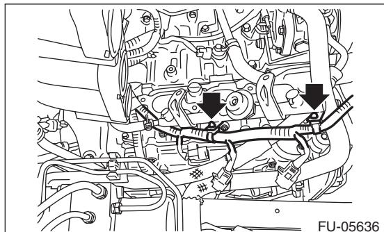
27) Remove the engine harness from the fuel injector pipe LH.
