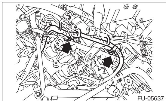
2) Install the engine harness to fuel injector pipe RH.
