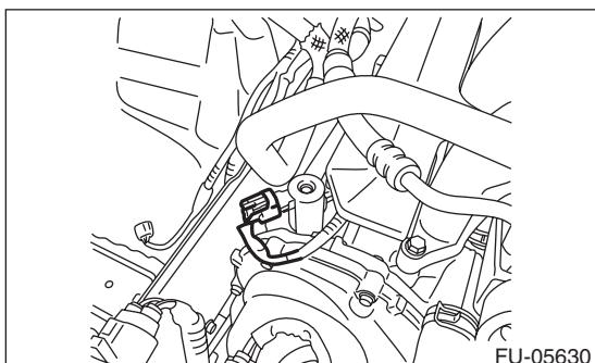
9) Install the bolts which hold fuel injector pipe LH to cylinder head.
