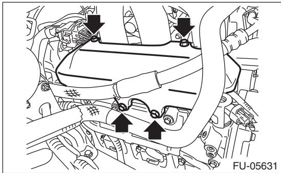
22) Disconnect #1, #3, and #5 fuel injector connectors.
