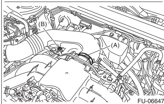
8) Remove the air intake boot assembly, and move it to the left side wheel apron.
