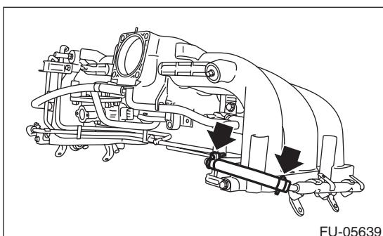
3) Remove the fuel pipe assembly.
