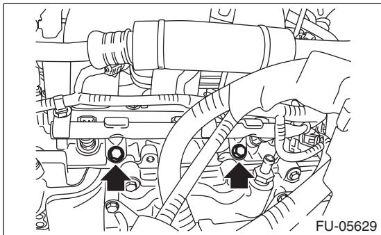
20) Disconnect the connectors of the intake oil flow control solenoid valve RH.
