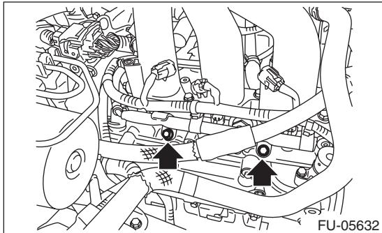
6) Connect #1, #3, and #5 fuel injector connectors.
