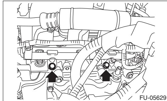
10) Connect the connectors of the oil temperature sensor, engine coolant temperature sensor and intake oil flow control solenoid valve LH.
