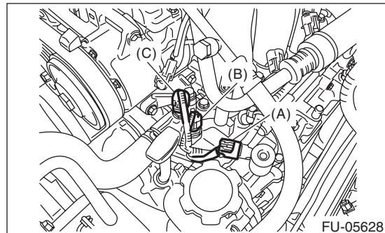
(A) Intake oil flow control solenoid valve LH
