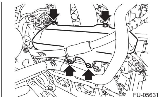
8) Connect the connectors of the intake oil flow control solenoid valve RH.
