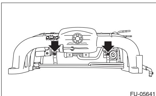
4) Remove the EGR valve. <Ref. to FU(H6DO)-42, REMOVAL, EGR Valve.>
