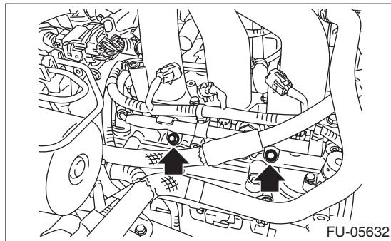
24) Remove the bolts which hold the intake manifold to the cylinder head.
