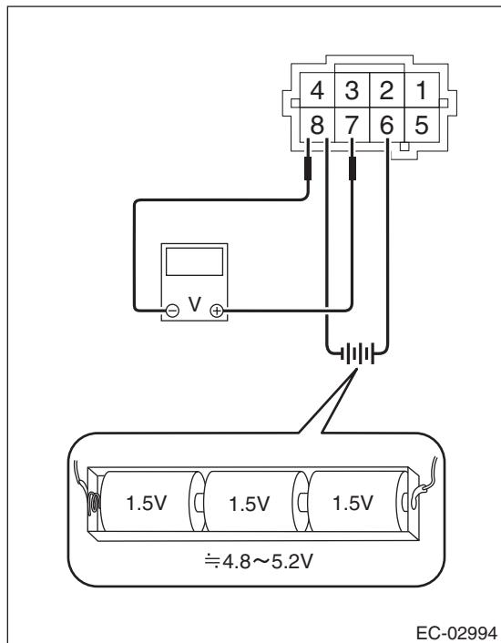
2) Check the voltage at a normal atmospheric pressure.
