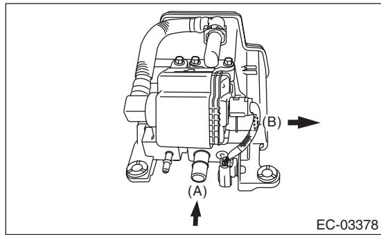
3) Connect the battery positive terminal to the terminal No. 5 and the battery negative terminal to the terminal No. 1. Check that air does not come out from (B) when air is blown into (A).
