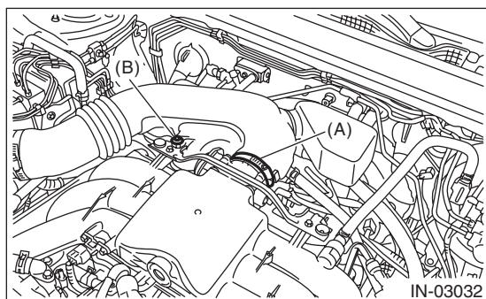
5) Disconnect the blow-by hose and remove the air intake boot assembly.
