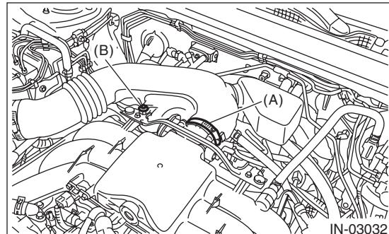
4) Tighten the clamp which connects the air intake boot assembly and air cleaner case (rear).
