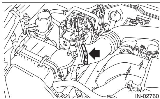
3) Loosen the clamp (A) which connects the air intake boot assembly and throttle body.
