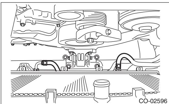
5) Install the radiator main fan & fan motor and radiator sub fan & fan motor. <Ref. to CO(H6DO)-22, INSTALLATION, Radiator Main Fan and Fan Motor. > <Ref. to CO(H6DO)-24, INSTALLATION, Radiator Sub Fan and Fan Motor. >
