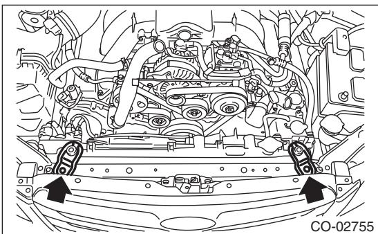
4) Connect the ATF radiator inlet hose and outlet hose.
