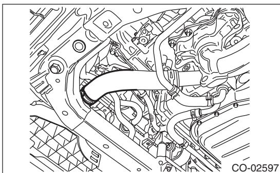
9) Connect the integrated connector of radiator main fan & fan motor and radiator sub fan & fan motor.
